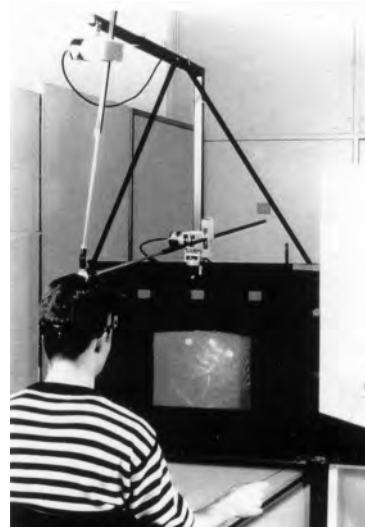
Figure 4.5: Coupling between the camera and the head of the observer during the experiment.
